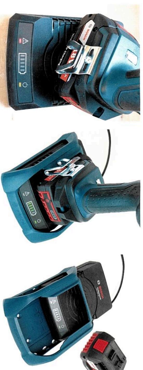
If the battery goes too far out of range the red warning light comes on
