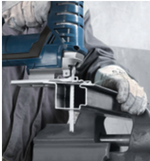
Thin-walled profiles up to 65 mm are easily cut with the T321 AF.
