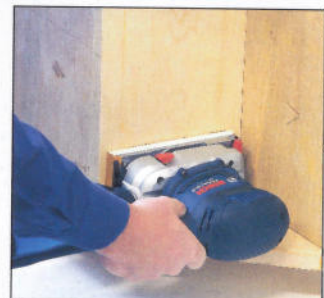
One advantage of traditional orbital sanders over random orbitals is that you can work right into corners
