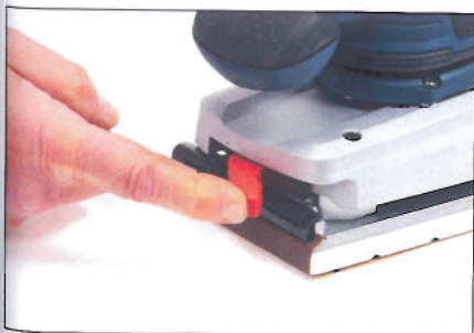
Then operate the front clamp to grip – and at the same time to tension – the sheet
