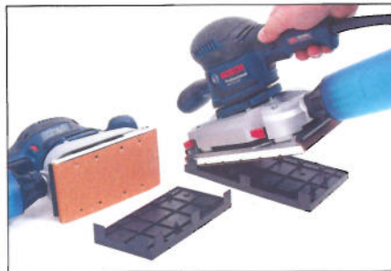
You need to buy a punch if you want to perforate your own abrasive sheets
