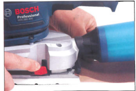
Depress the large rear clamp to load the first end of the abrasive sheet
