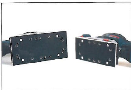
There's quite a difference in size of the sanding plates between the two models
