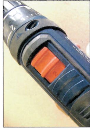
The speed selecting switch is conveniently located on top of the body casing
