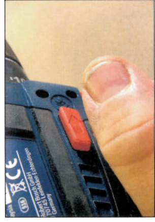
The forward and reverse switch is comfortably positioned on the side of the drill
