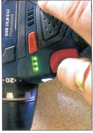
The LED indicator on the side gives an accurate indication of the charge level
