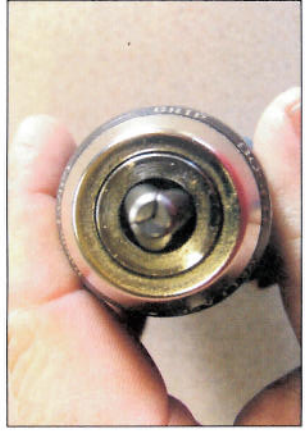
The keyless chuck closes down to zero, so it will hold small drill bits securely
