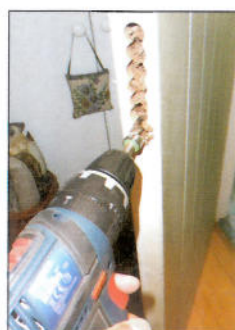
A single LED fires a beam of light from the base just in front of the chuck
