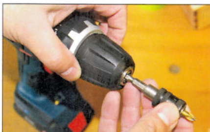
The single-sleeve chuck will take bits up to 13mm in diameter
