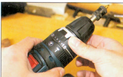
The torque collar controls the drill function. The rear collar is for hammer work
