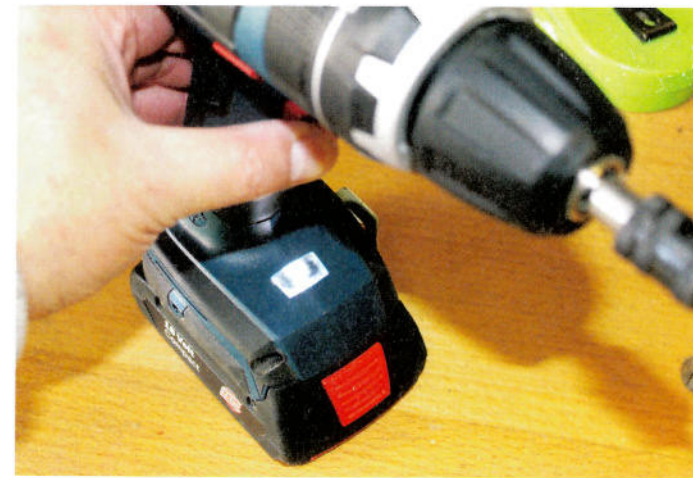
▲ A single LED fires a beam just in front of the chuck
