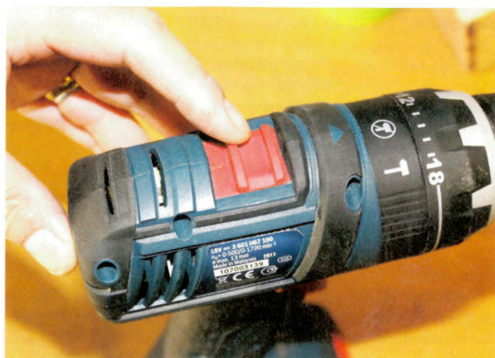
▲ This large slider controls the gearbox for speed changes
