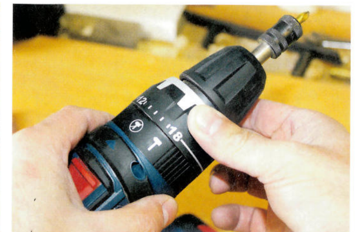
▲ The torque collar also controls the drill function; the rear collar is for hammer work
