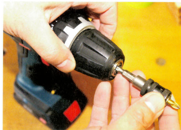
▲ The single-sleeve chuck will take up to 13mm-diameter bits
