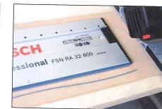
Once the first cut has been completed on a sacrificial board, the saw is ready for proper use. Note the offcut of protective strip
