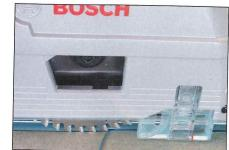
The first cut will trim the protective strip to a perfect fit. The clear adjustable dust shield increases extraction efficiency
