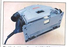
The black strip on the underside of the saw is the low-friction groove which engages with the rail and ensures a smooth action
