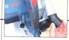
The exhaust port swivels for ease of use. The knob on the sole plate adjusts the grip on the rail
