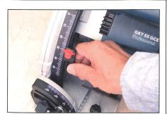
The depth of cut is set using the large scale. The smaller angle scale for setting bevel cuts is at the front of the saw body
