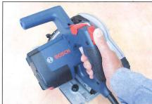
The thumb-operated lock button in action on top of the handle. Note the red spindle-lock cover positioned forward of it
