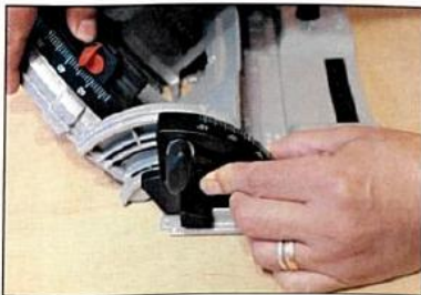
You can override the standard bevel settings with the small buttons on the protractor scales
