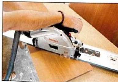
The saw operates smoothly on repeat miter cuts using the bevel setter
