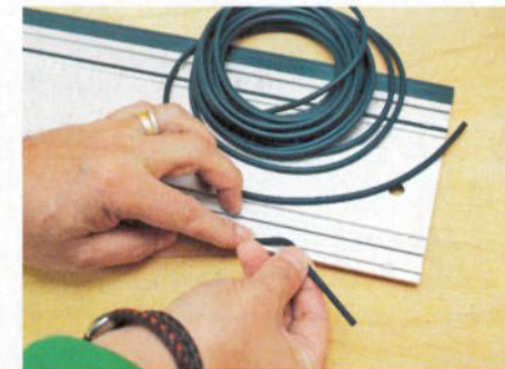
▲ These replaceable round rubber inserts work like a charm to hold the rail
