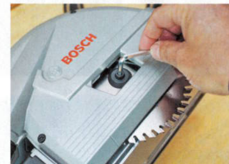
▲ ...which sets the blade at the correct position to gain access to the blade-retaining flange
