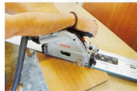
▲ The saw operates smoothly on bevel cuts using the bevel setter
