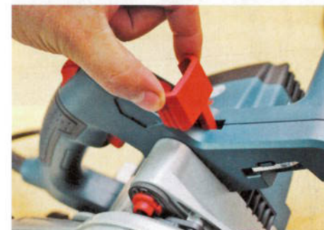
▲ Blade changing is a cinch; lifting this lever engages a locking pin...
