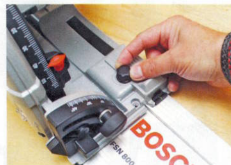
▲ The base can be adjusted to fit the rail for a perfect fit using the dials on the top of the base
