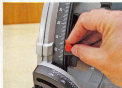
▲ Plunge depths are set on this scale; the cursor rotates to indicate the depth on or off the rail
