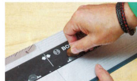
▲ To connect the rails the wide flat plate keeps them perfectly aligned; the plate holds can be nipped up with a coin and can stay on board when not required
