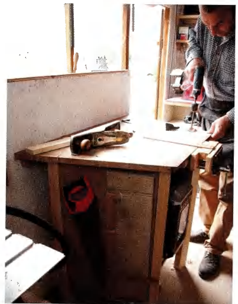
Hex Nick is trying to see if he can survive in the shed with only a hex-drive Bosch 10.8V cordless driver, using a small Trend chuck when necessary to reduce the amount of space used up with too many tools. With the Bench Blade in position and a home-made stop in the vice you can plane short boards on a small vice easily (below)
