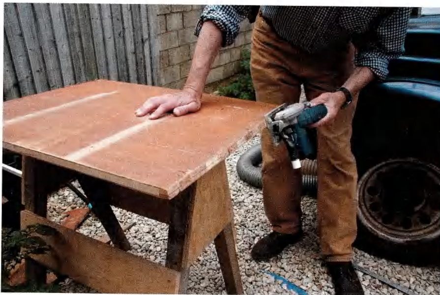
Assembly Cutting the angles on the back board which holds the bench together (above). It wasn't easy, and if the bench is any use Nick will probably have another go to tidy up the joints. Drilling a hole for a Bench Blade (left)
