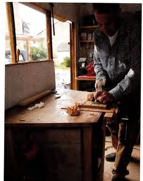
Hex Nick is trying to see if he can survive in the shed with only a hex-drive Bosch 10.8V cordless driver, using a small Trend chuck when necessary to reduce the amount of space used up with too many tools. With the Bench Blade in position and a home-made stop in the vice you can plane short boards on a small vice easily (below)
