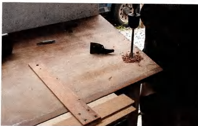
Assembly Cutting the angles on the back board which holds the bench together (above). It wasn't easy, and if the bench is any use Nick will probably have another go to tidy up the joints. Drilling a hole for a Bench Blade (left)
