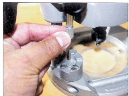
The turret post has a small adjuster screw for fine-tuning the cut
