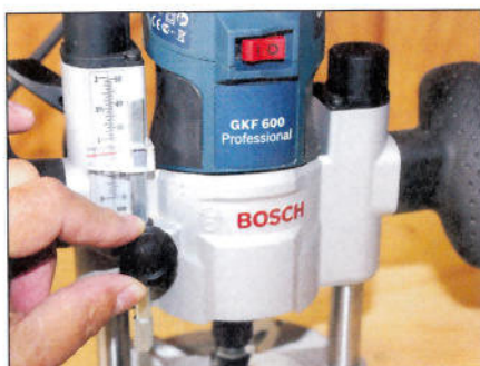
After adjusting the turret post, you secure it with this locking knob
