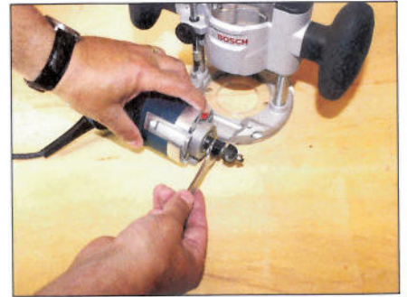
You have to remove the body from the base to change cutters
