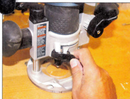
Lock the base to the motor housing with this easy-to-operate toggle
