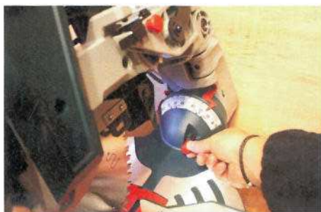
▲ There are index points for compound cuts, locked with this pin
