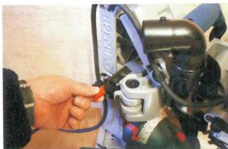
▲ The glide action can be locked with this pivoting peg for standard chop cuts
