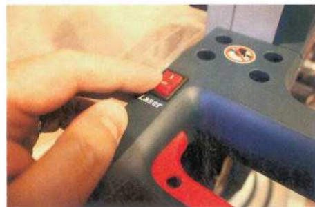
▲ The twin laser can be switched off if necessary
