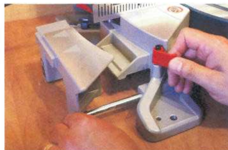
▲ Small cam levers lock the pull-out supports
