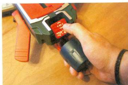
▲ You rotate the turntable by unlocking this central button
