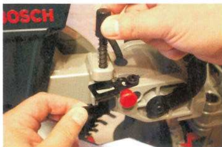
▲ Trench cuts are set using this threaded rod and stop
