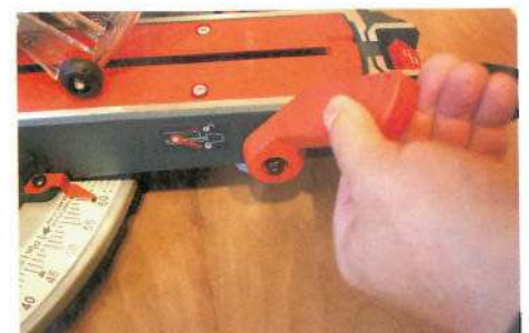
▲ The dual tilt function uses a combination of this lever...
