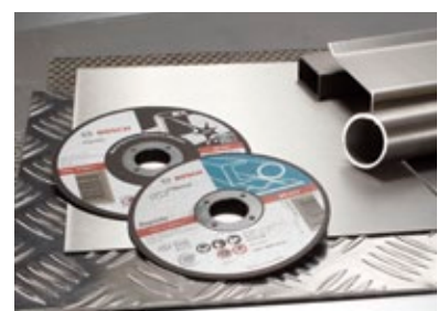
Lifetime of a cutting disc: cut workpiece area divided by the consumption area of the disc (mm 2 /mm 2 ) = G. The higher the G value, the longer the lifetime of the disc. Tests by Bosch in 10×30 mm inox, with 230×2.5 mm Best for Inox cutting disc, with 2600 watt angle grinder.
